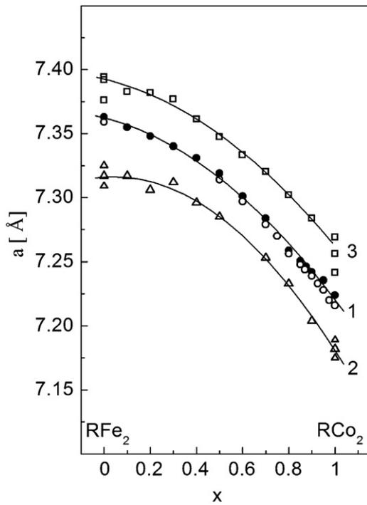
**Fig. 1.** The unit cell edge  $a$  (curve 1) observed for the  $Y(Fe_{1-x}Co_x)_2$  intermetallics (300 K). The literature data (open points) are added [1,25]. Additionally are presented data for  $Dy(Fe_{1-x}Co_x)_2$  (curve 2) [1,17,26] and  $Gd(Fe_{1-x}Co_x)_2$  (curve 3) [1,15,16].
