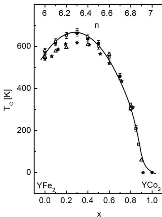
**Fig. 5.** The Curie temperature  $T_C(x)$  of the  $Y(Fe_{1-x}Co_x)_2$  series (black points – electrical resistivity measurements, open points – Mössbauer effect measurements). Open squares, triangles and stars correspond to literature data [25,40,41]. Upper axis shows number  $n$ .
