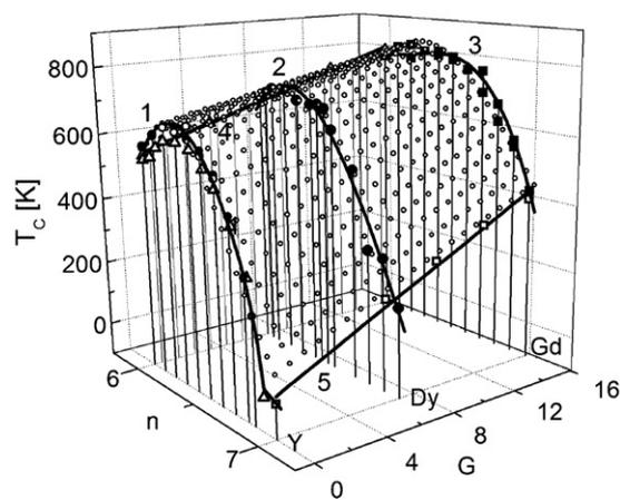
**Fig. 6.** The covering function  $T_C(n, G)$  (marked by small open points) based on the series:  $Y(Fe_{1-x}Co_x)_2$  (curve 1),  $Dy(Fe_{1-x}Co_x)_2$  (curve 2) [17],  $Gd(Fe_{1-x}Co_x)_2$  (curve 3) [15,16],  $(Y_{1-x}Gd_xFe_2)$  (curve 4) [46] and  $(Y_{1-x}Gd_xCo_2)$  (curve 5) [47].
