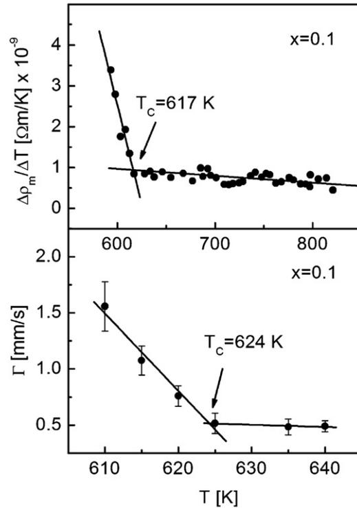
**Fig. 4.** The exemplary  $\Delta\rho_m/\Delta T$  ratio (upper case) and the half-width  $\Gamma$  of the Mössbauer line (lower case) as functions of temperature  $T$  are presented for the  $Y(Fe_{0.9}Co_{0.1})_2$  compound in the Curie temperature region. The intersection of lines determines the Curie temperature  $T_C$ .
