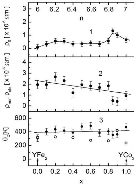
**Fig. 3.** The residual resistivity  $\rho_0$  (curve 1), the asymptotic magnetic resistivity  $\rho_{m\infty}$  or  $\rho_{sf\infty}$  (curve 2) and the Debye temperature  $\theta_D$  (curve 3) as functions of the composition parameter  $x$  for the  $Y(Fe_{1-x}Co_x)_2$  compounds. The literature Debye temperatures  $\theta_D$  (open points) are added [31].
