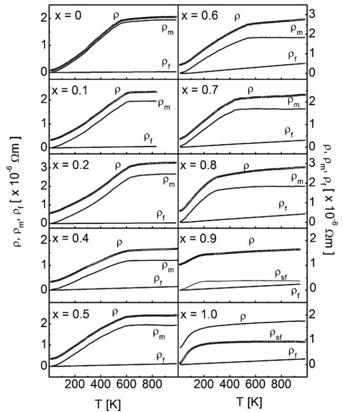
**Fig. 2.** Electrical resistivities: the total  $\rho$ , the phonon  $\rho_f$  and the magnetic  $\rho_m$  or  $\rho_{sf}$  observed against temperature for the  $Y(Fe_{1-x}Co_x)_2$  compounds.
